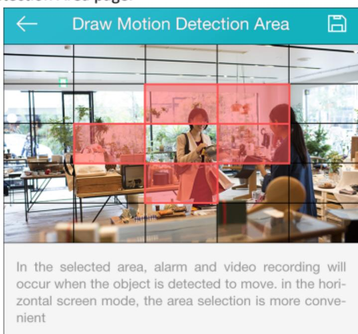
**Figure 12-3 Draw Motion Detection Area**
